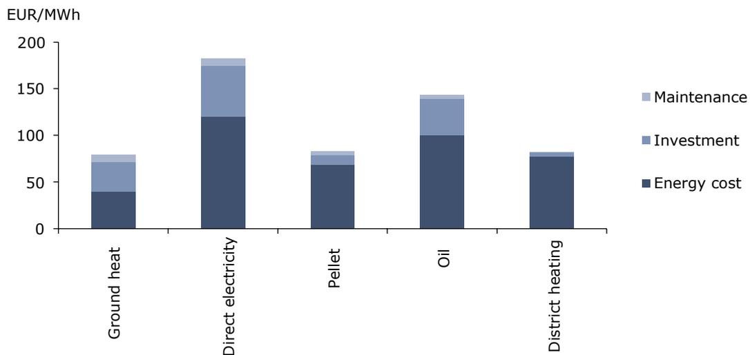
The example building in the LCOE calculation is a block of flats with an annual heating need of 469 MWh. The LCOE calculations include investment costs, operating costs and energy costs, i.e. fuel costs and electricity costs. The interest rate used is 3%.
