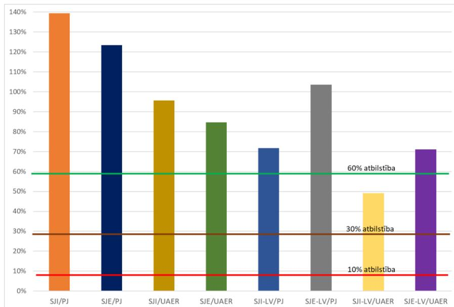
**Figure 26. Electricity interconnectivity level of Latvia in 2018**
