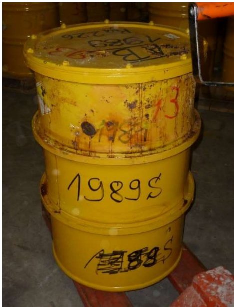
Aging drum with radioactive waste from 1981
