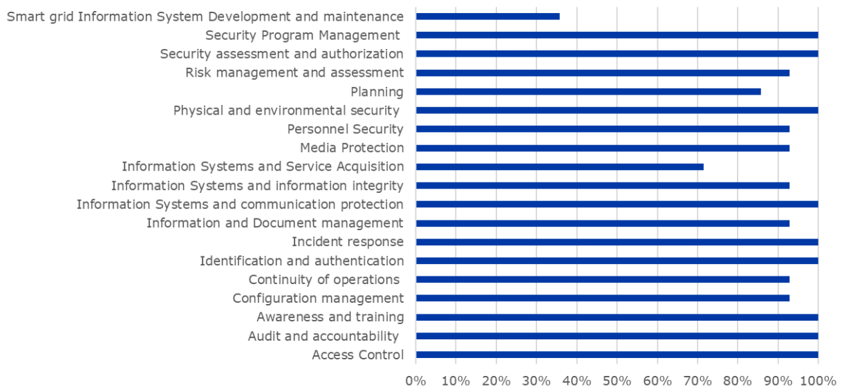
Figure 12: Type of measure classes applied by system operators [project survey, based on NISTIR 7628 classification]
