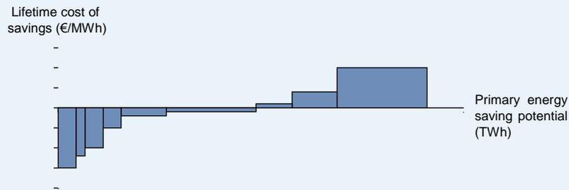
Figure 1-1: Illustrative energy efficiency cost curve
