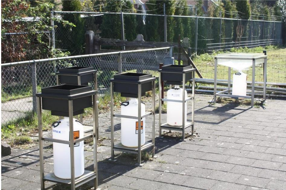
Figure 2. RIVM Dry/wet deposition collectors
