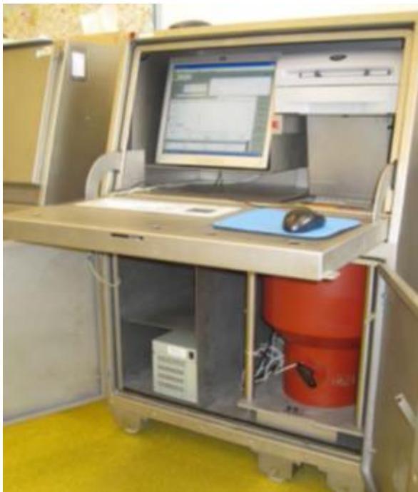
**Figure 5. Fixed monitoring station for radioactivity in food and feed**
