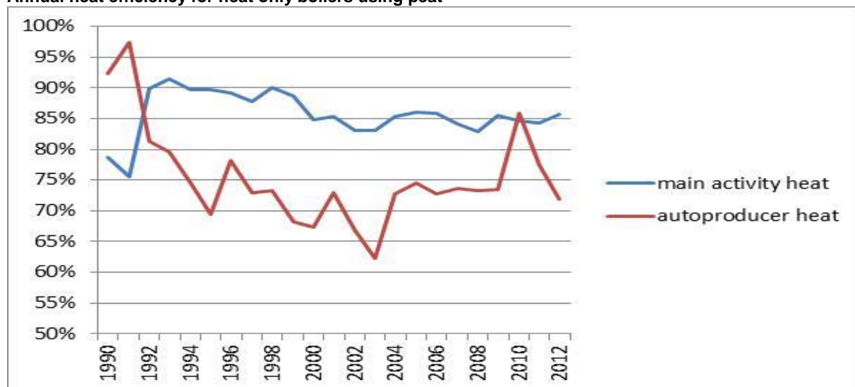
Annual heat efficiency for heat only boilers using peat
