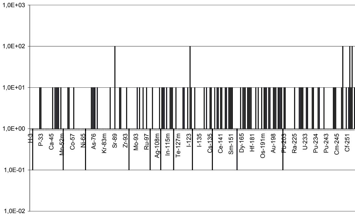
Figure 4.1: Ratios of values in RS-G-1.7 and RP 122 Part I (final values), excluding radionuclides termed “natural” in RS-G-1.7
