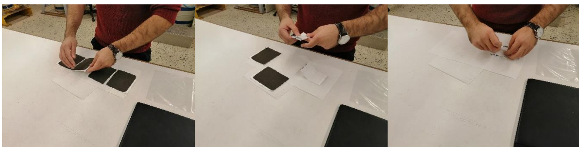
Figure 19. The air sample filter (8"x10" glass fibre) is folded to geometry of 5.08 \times 6.35 \times 0.9 \text{ cm}^3 in preparation for measurement by gamma ray spectrometry.
