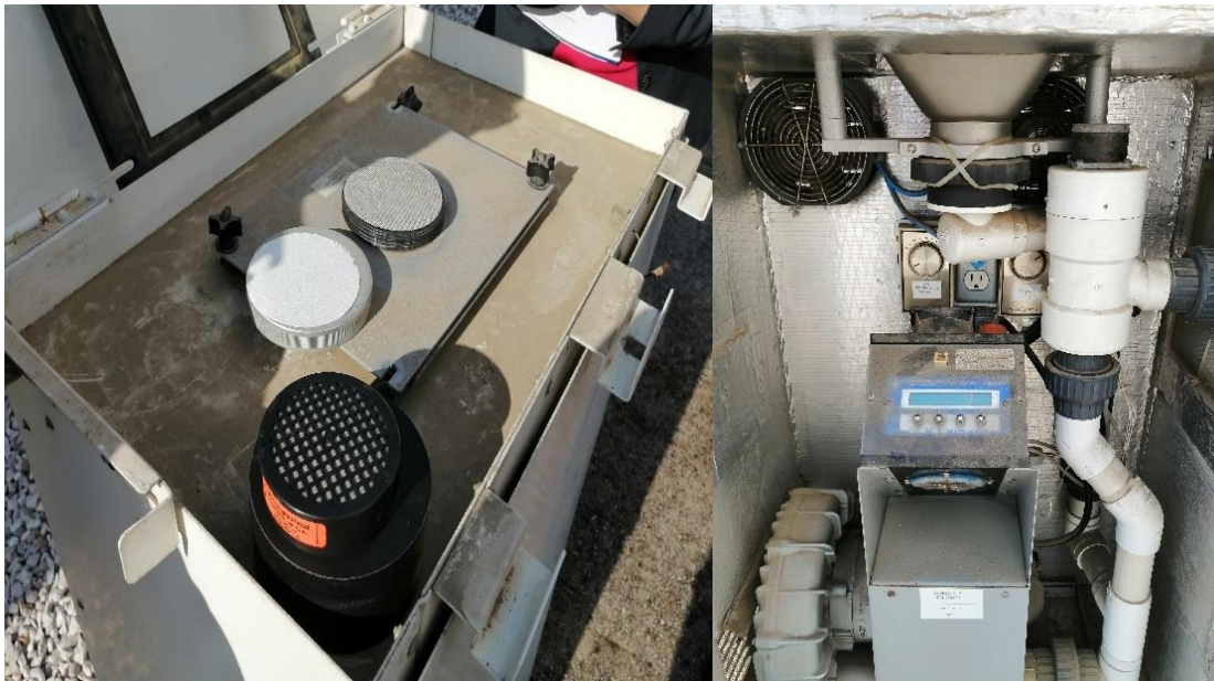
Figure 17. NTUA high volume air sampler and optional iodine cartridge
