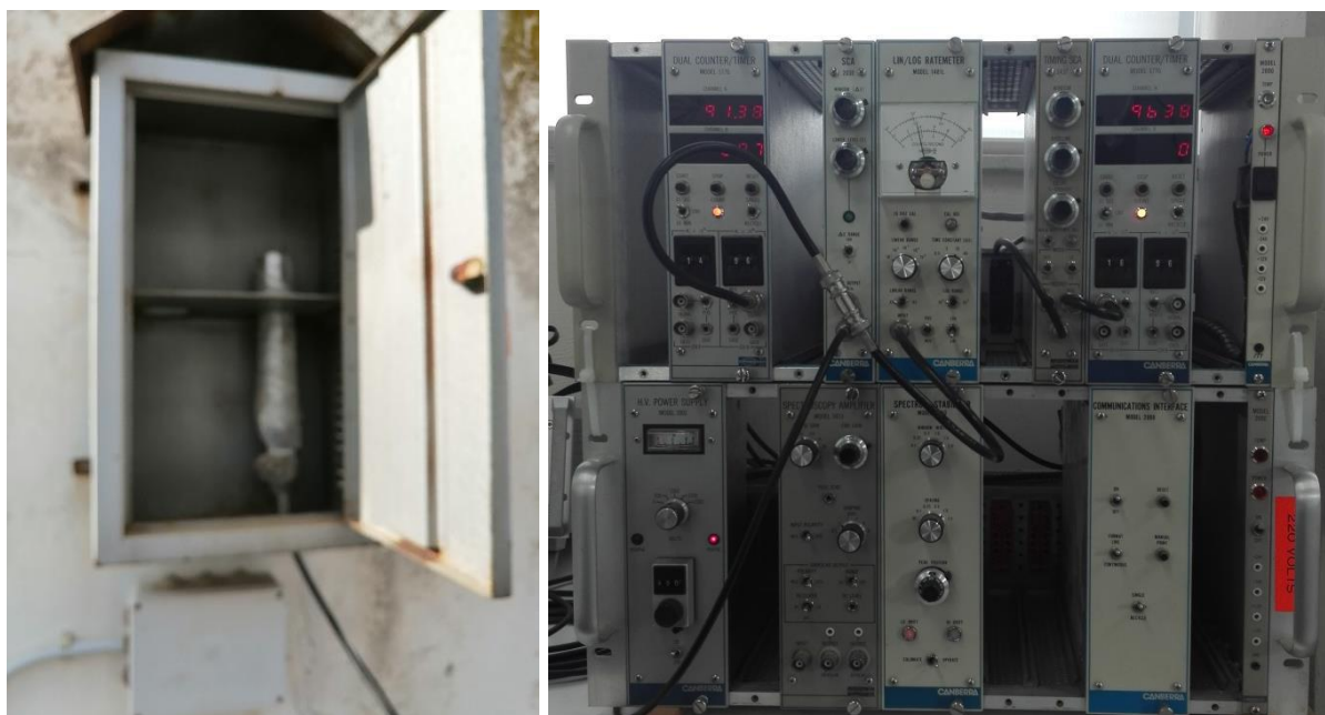
Figure 16. NTUA early warning on-line system for Cs-137 radioactivity in air
