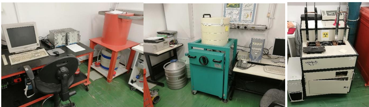
Figure 15. ERL laboratory counting equipment (HPGe gamma spectroscopy and total alpha/beta)
