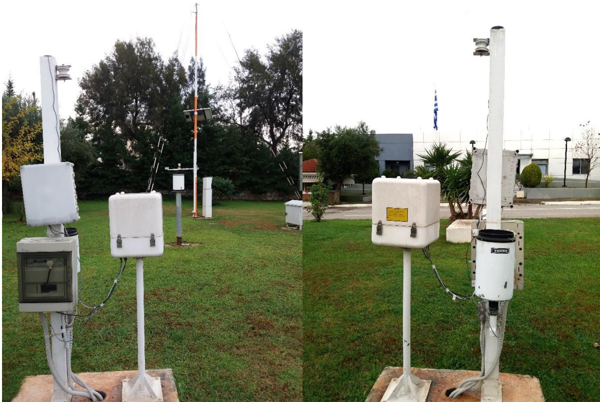
Figure 5. Ambient dose rate monitoring station at Hellinikon, Athens (part of the Telemetric Radioactivity Monitoring Network)
