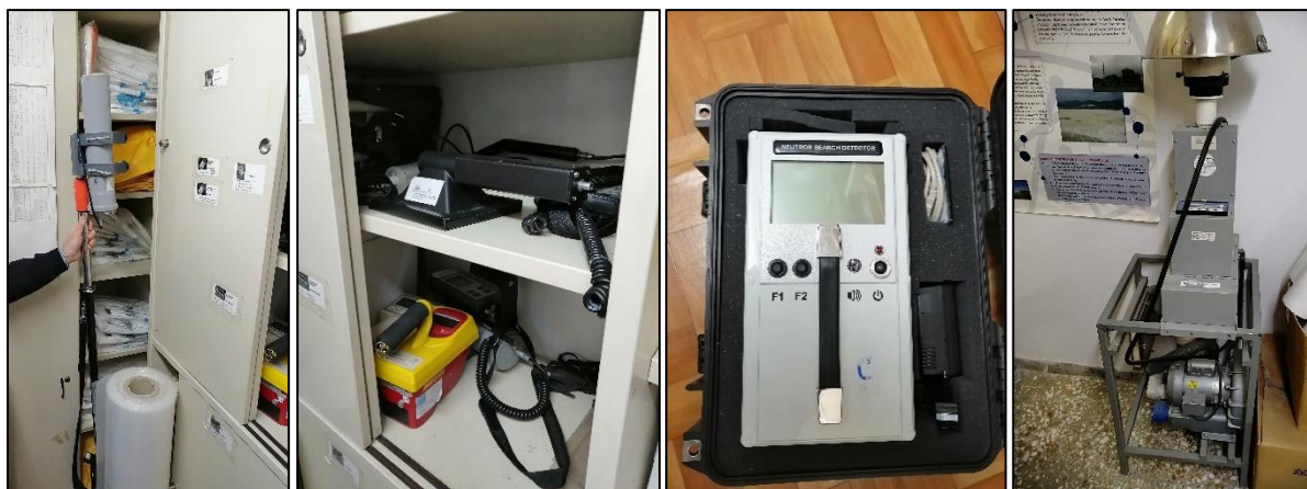
Figure 14. EEAE mobile monitoring equipment (Nal telescopic probe, dose rate & contamination monitors, neutron survey monitor, portable air sampler)
