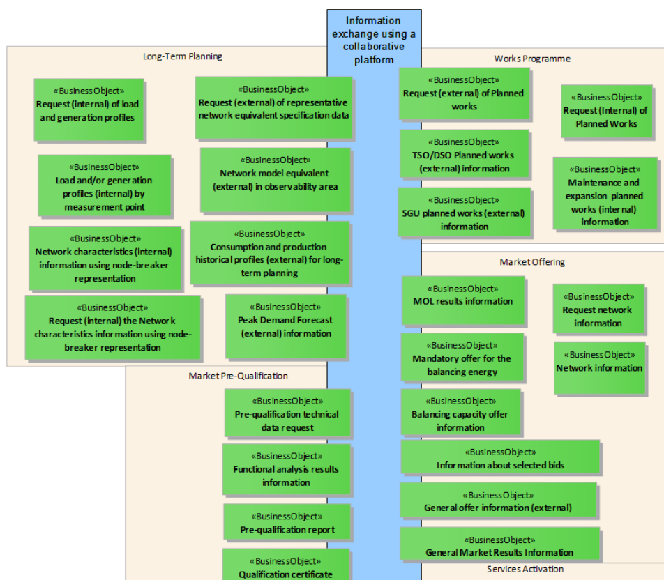
Figure 34: CIM repository – UML repository for Business Objects (example from TDX-ASSIST UML repository)
