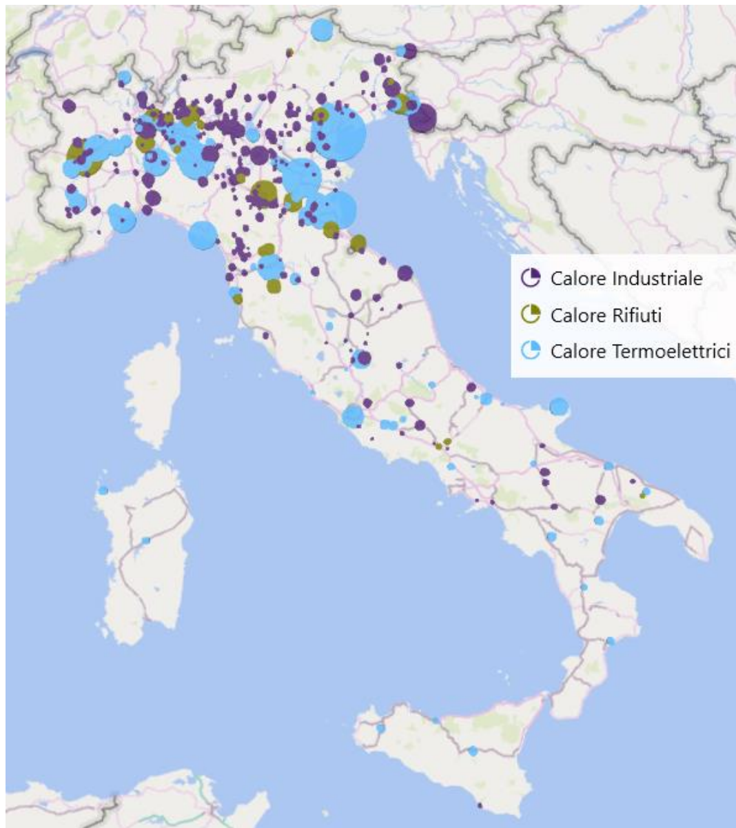
Figure 107: Technical potential map of heat recovery in district heating networks from industrial, thermal power and waste plants
