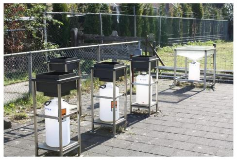
Figure 2. RIVM Dry/wet deposition collectors
