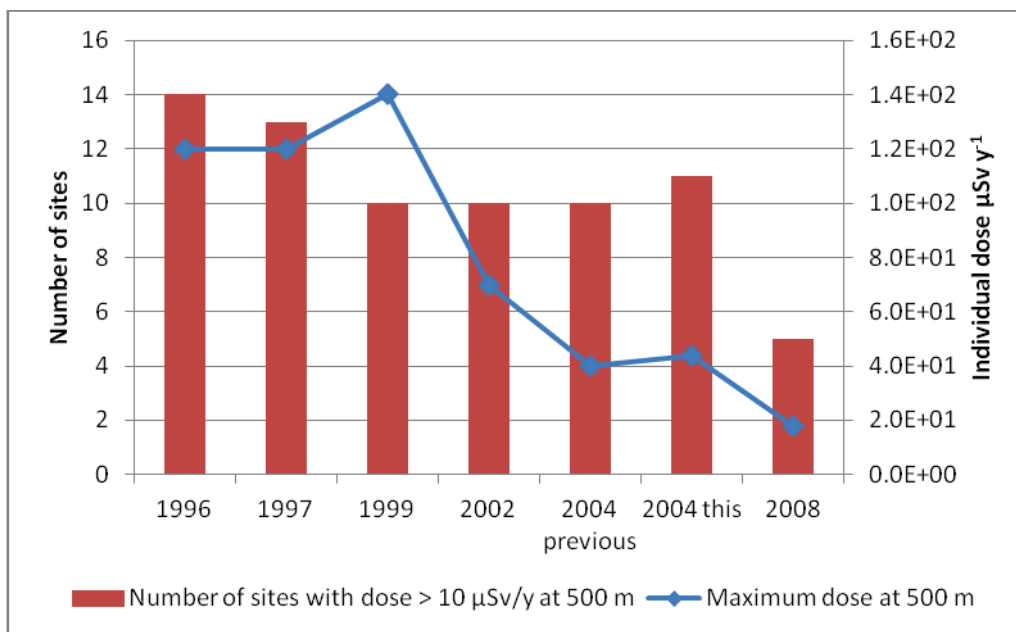
Figure 6: Maximum dose received by a representative person living 500 m from operating nuclear power stations ( \mu\text{Sv y}^{-1} ) as a result of reported atmospheric discharges and the number of sites where the dose is greater than 10 \mu\text{Sv y}^{-1}
