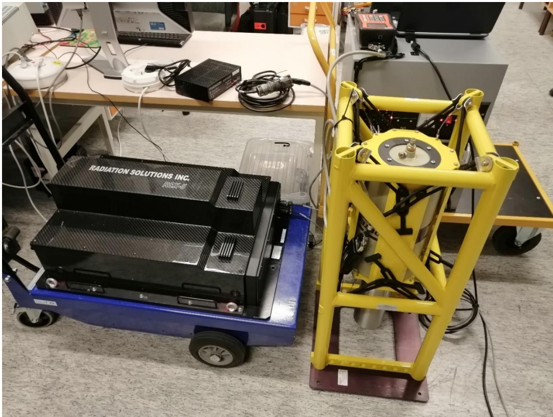
Figure 10. NaI and HPGe detectors of the SGU for airborne monitoring
