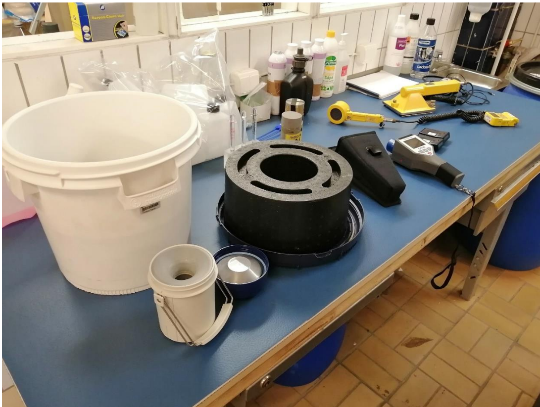
Figure 12. Civil protection CBRN detection team equipment for securing small radiation sources and for monitoring radiation
