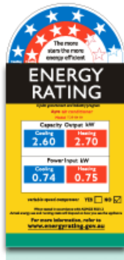
Figure 6-2 - Generic energy label in Australia
