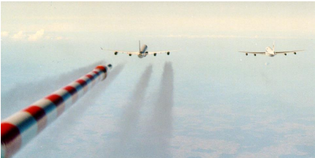
Demonstration of the influence of exhaust gas temperature on contrail formation. An older B707 without contrail (right, hotter exhaust gas) alongside a modern A340 with contrail (left, cooler exhaust gas); Photo taken from the cockpit of DLR's research aircraft Falcon. (Schumann et al., J. Aircraft (2000)).
