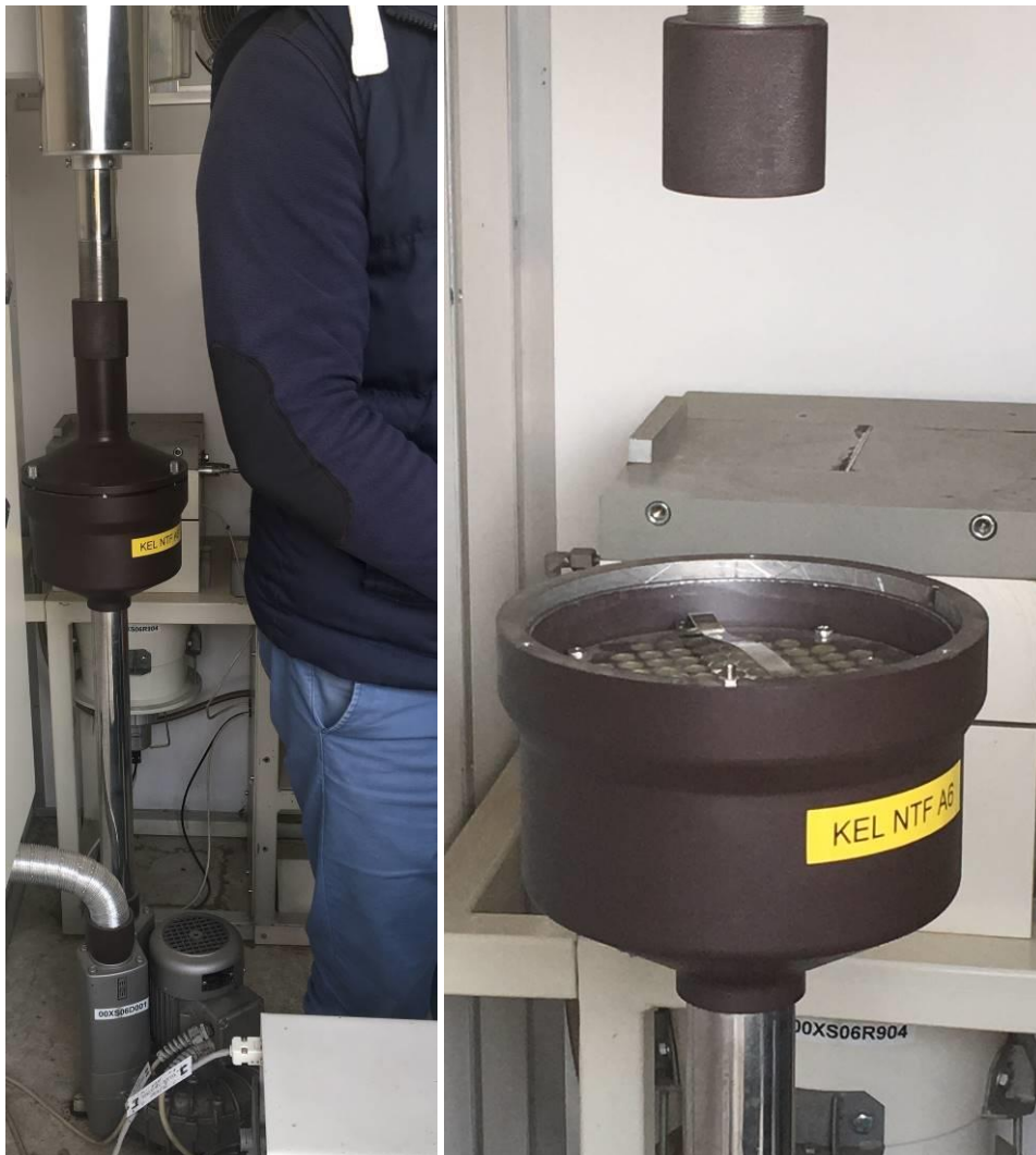
Figure 16. The large volume air sampler (left – assembled, right – taken apart)
