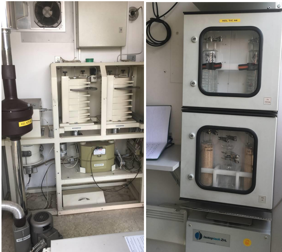
Figure 2. Left side: large and small volume air samplers inside a combined sampling unit. Right side: carbon (above) and tritium (below) samplers
