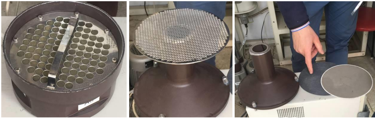
Figure 17. The large volume air sampler disassembled. On the left – filter at the bottom of the sampler, mesh in the middle, on the right – fine filters situated on the top part.
