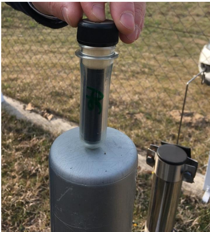
Figure 7. Al 2 O 3 containing capsule for monthly background dose integration
