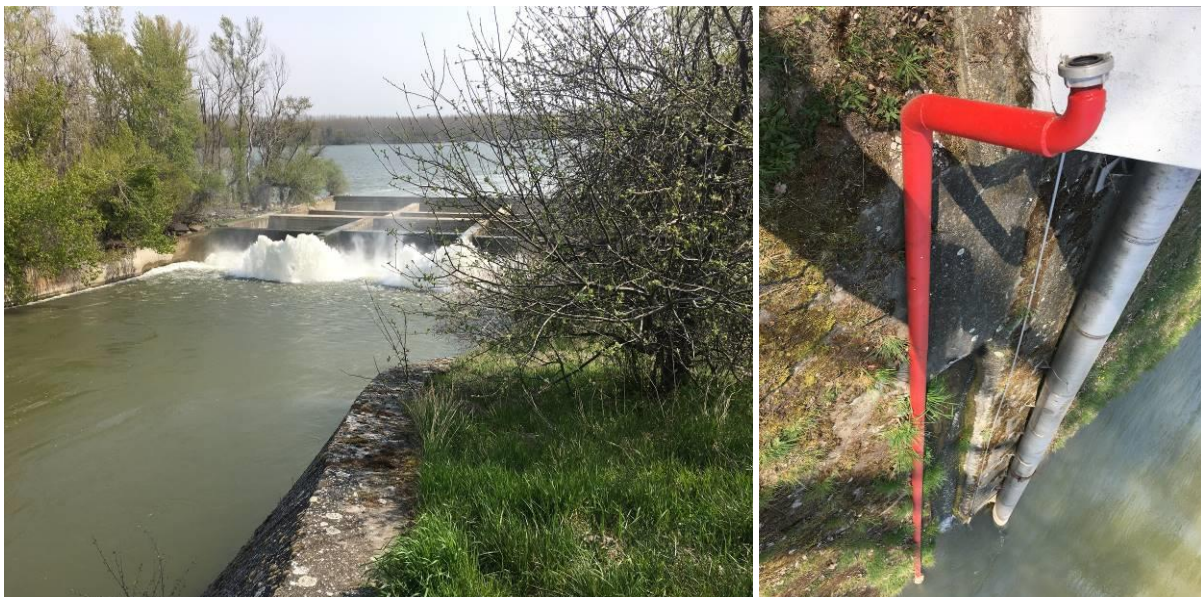
Figure 13. The warm channel and sampling tubes (grey leading to V2 monitoring station)
