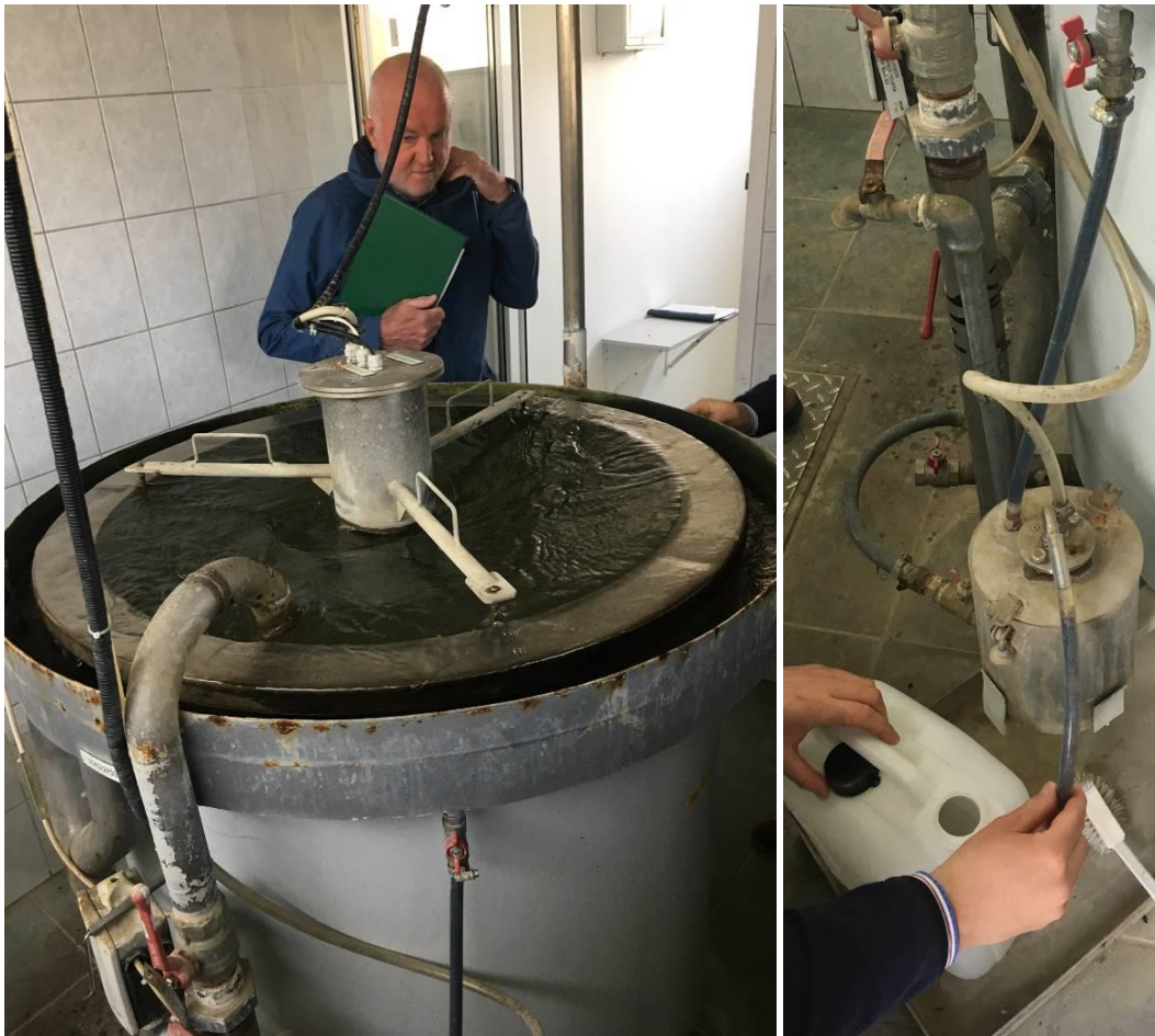
Figure 14. Left: continuous monitoring of the water flowing to Danube River; right - sampling in action
