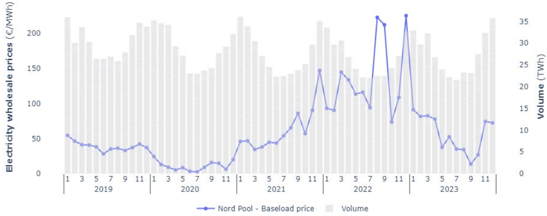
Figure 41 – Monthly electricity exchange traded volumes and the average day-ahead wholesale prices in Northern Europe
