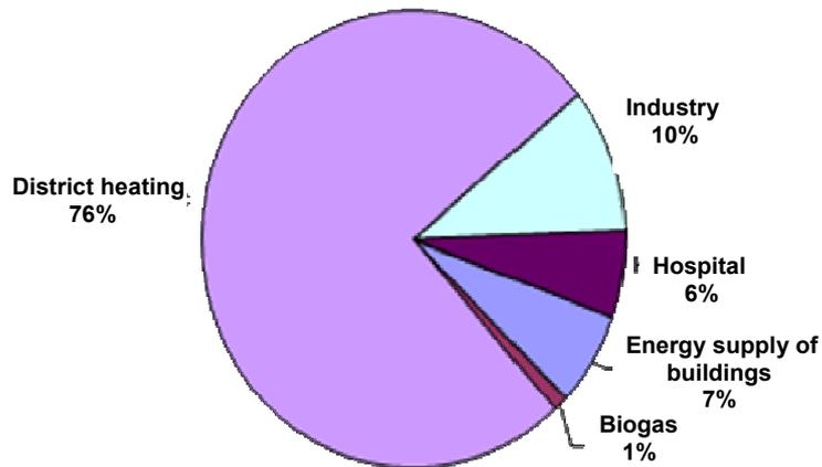
Analysis of the fields of application shows that 76% of all installed capacity – i.e. over 310 MW electric capacity – is installed in the district heating systems. This is because district heating services are highly widespread in Hungary.
