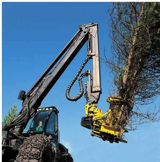
Harvesting of small-size trees by an accumulative harvester head, which collects the trees. Timberjack.
