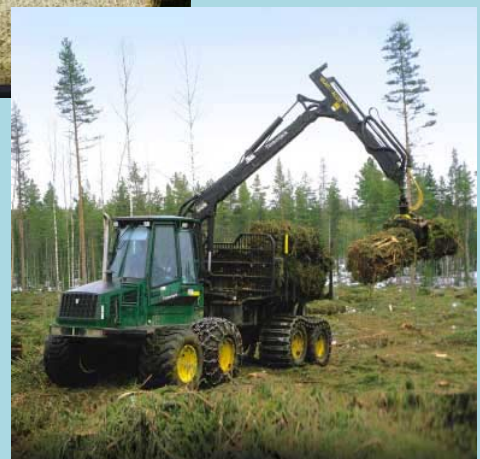
Forest fuel supply is based on bundling of logging residues. The bundles are delivered by classic timber lorries to the plant and crushed on site at CHP plant. Timberjack.
