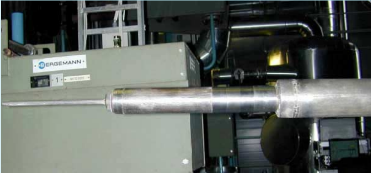
Deposit formation test probe for full-scale boilers before and after a test period in a superheater area. VTT Processes.
