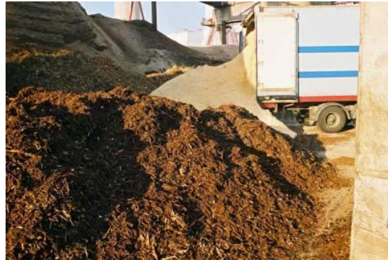
Bark, sawdust and the mixture of bark, sawdust and logging residue chips in the fuel yard of a large-scale power plant. VTT Processes.
