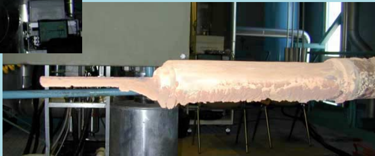
Deposit formation test probe for full-scale boilers before and after a test period in a superheater area. VTT Processes.
