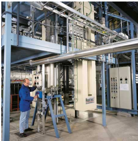
Bubbling bed pilot reactor for testing of fuels and combustion behavior. VTT Processes.
