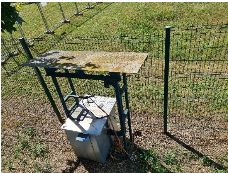
Figure 10. High volume air sampler at the IOS
