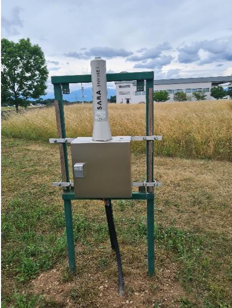
Figure 42. Spectrometric station SARA at the Research Reactor premises
