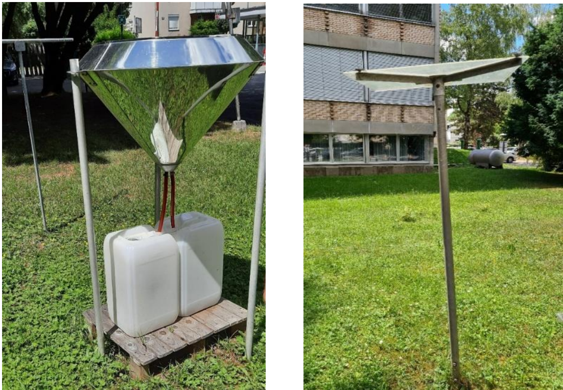
Figure 14. Atmospheric wet deposition (left) and dry deposition collectors at the JSI (right)
