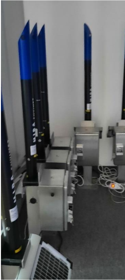
Figure 39. New MIRA GDRs stored at the SNSA premises
