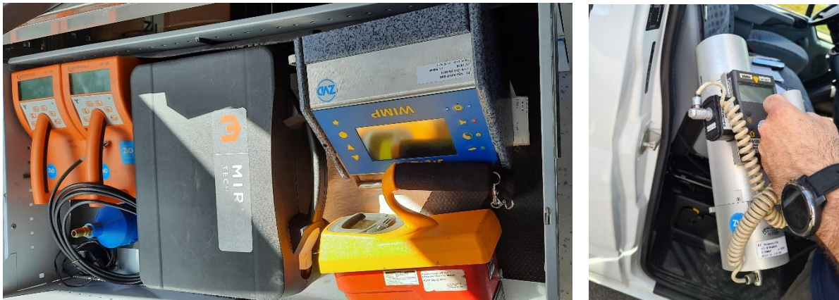
Figure 45. Handheld dose rate/contamination monitors and a plastic scintillator in the IOS environmental monitoring vehicle
