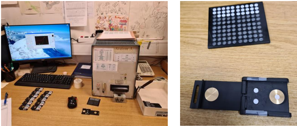
Figure 7. TLD reader at the TLD laboratory of the JSI (ICMIS)
