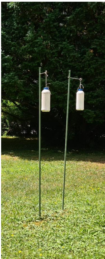
Figure 6. TLD dosimeters in plastic bottle housing at the JSI garden
