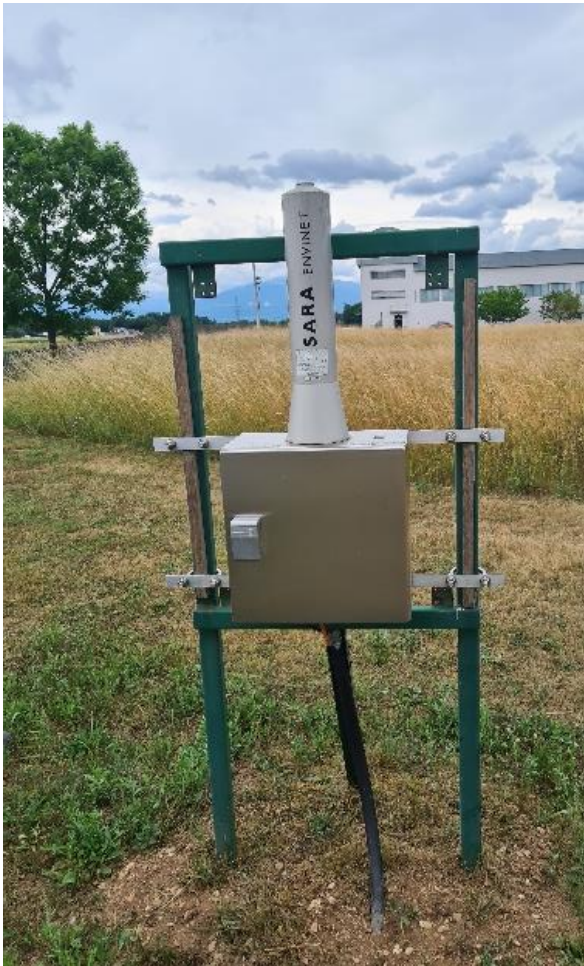
Figure 4. ENVINET SARA – fixed spectroscopic gamma detector, at the Research reactor premises
