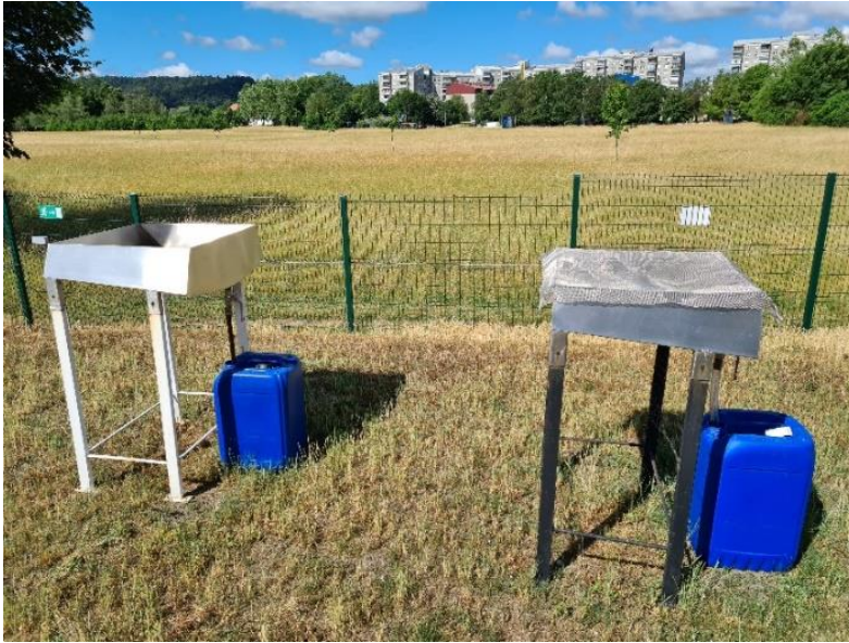
Figure 15. Atmospheric dry and wet deposition collectors at the IOS
