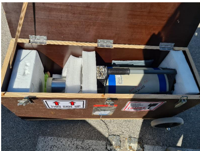
Figure 47. Mobile HPGe gamma spectrometer in the IOS environmental monitoring vehicle
