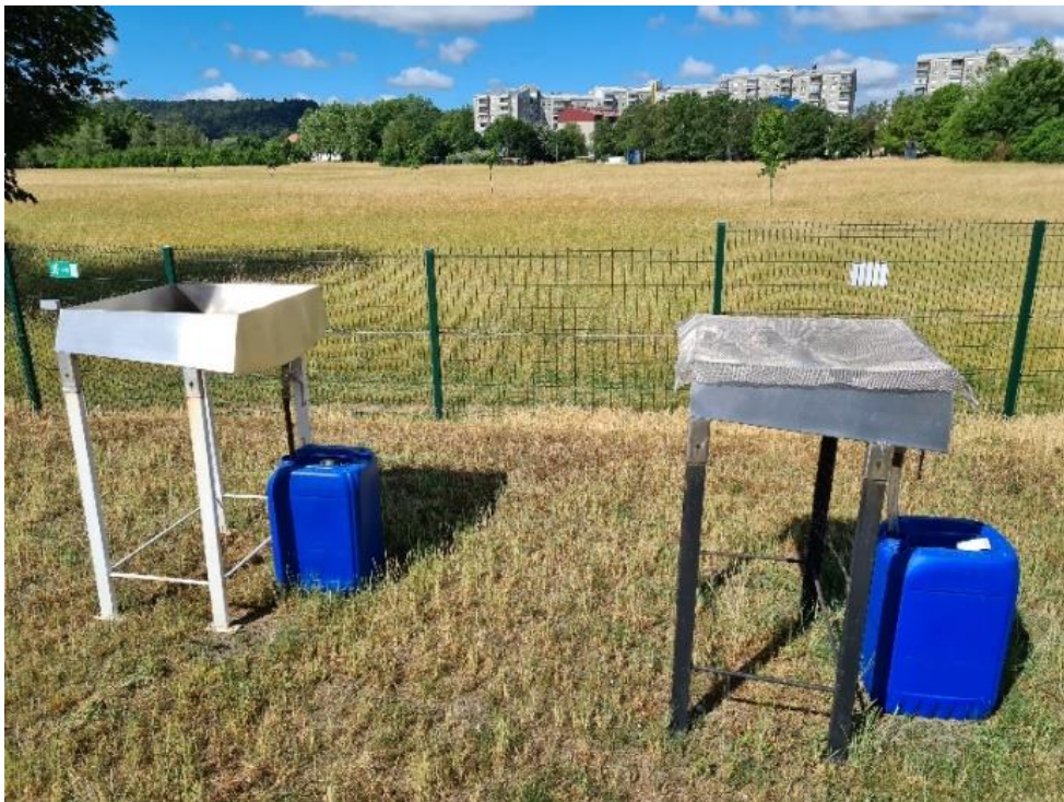
Figure 37. Dry and wet deposition collectors at the IOS
