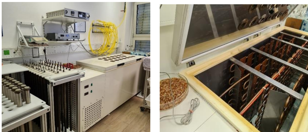
Figure 30. Tritium electrolytic enrichment system at the JSI
