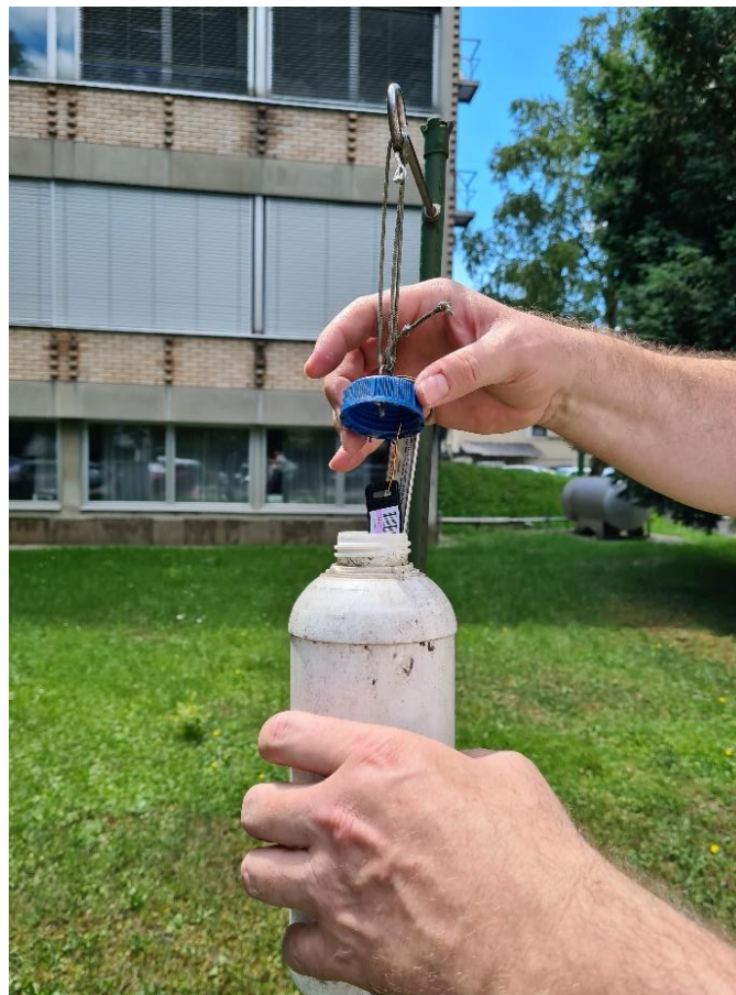
Figure 6. TLD dosimeters in plastic bottle housing at the JSI garden
