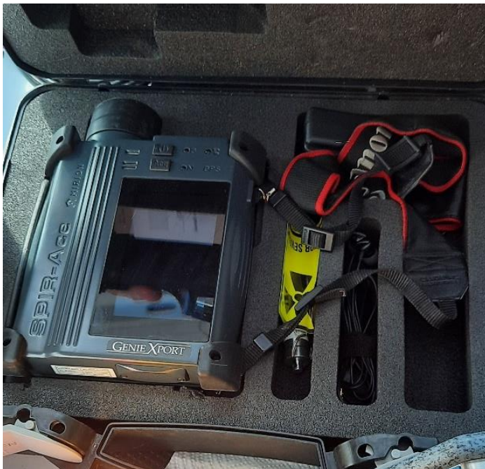
Figure 46. Radio Isotope Identification Device SPIR-Ace in the IOS environmental monitoring vehicle
