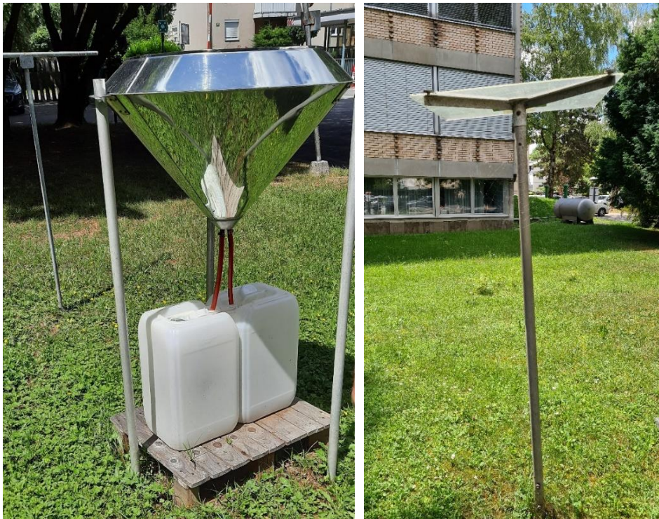
Figure 38. Atmospheric dry and wet deposition collectors at the JSI
