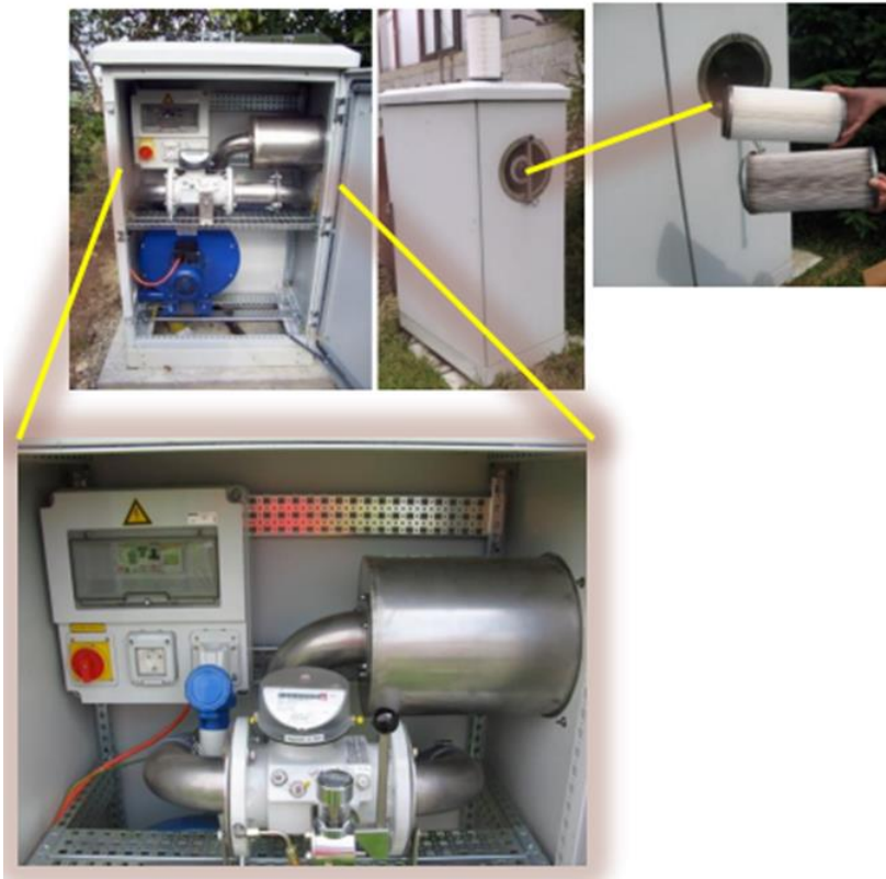
Figure 9. High volume air sampler of the JSI
