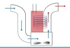
Airflow in an electric heater; Fresh, outside air is sucked in by a fan and led through a heating chamber. In the heating chamber a heating element is placed which heats the cold air. This warm air is then released to the indoor environment.
