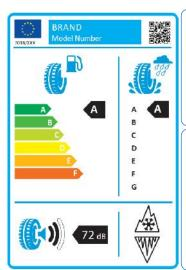
New proposed label for tyres, to be used from 2020, showing the label class for fuel efficiency, the label class for wet-grip, the noise-emission level, and the symbol for use on snow or ice, if applicable.
