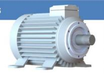
The efficiency of electric motors is indicated using classes (IE1, IE2, IE3) according to IEC600034-30: 2008. In the same class, the efficiency depends on the motor output power, e.g. an IE3 motor of 1 kW output has an efficiency around 85%, but an IE3 motor of 100 kW output has an efficiency around 96%.
