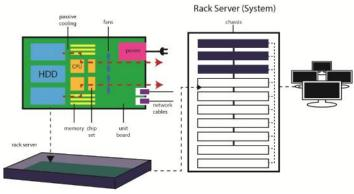
Rack servers are stand-alone devices, comprising all necessary components to operate. The rack servers can be stacked in a standardized U-rack (hence their name), for ease of management and interconnection for combined computing power.
