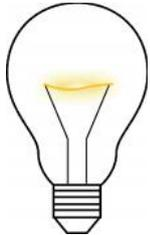
GLS = General Lighting Service: the classical 'Edison' filament lamp. When an electric current is made to pass through a thin metal wire (the 'filament'), the metal opposes the current flow (electrical resistance) and as a result heats up and starts to glow (becomes 'incandescent'), emitting electro-magnetic radiation of which a small part is visible, called light. Dominated sales until 2008-2010, but now phased-out due to Ecodesign. Efficacy around 10 lm/W.
