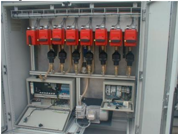
Picture 13. Air sampler with a filter for each day of the week
