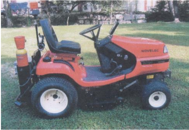
Picture 3. Measurement device used for the contamination control of the pathways
