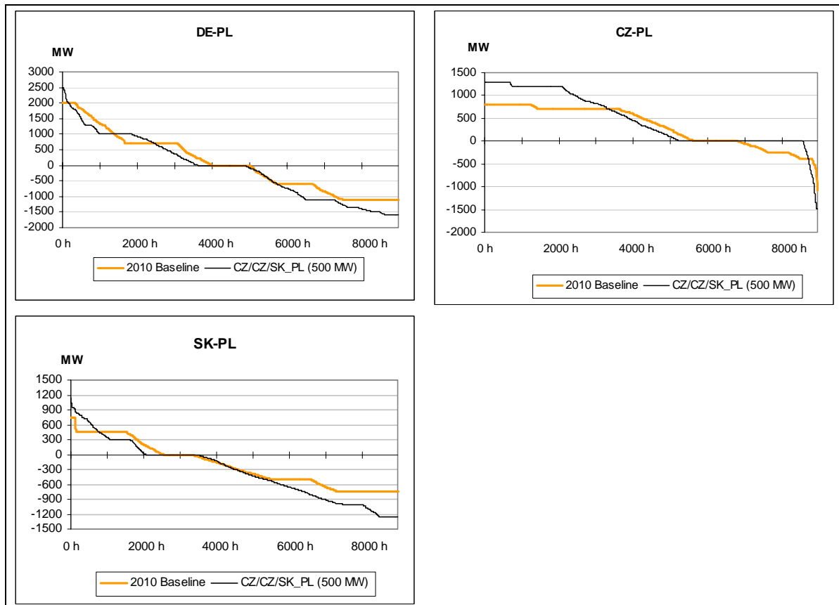
Figure 45: Changing flow patterns in case of increased import capacities CZ/CZ/SK \leftrightarrow PL (500 MW)
