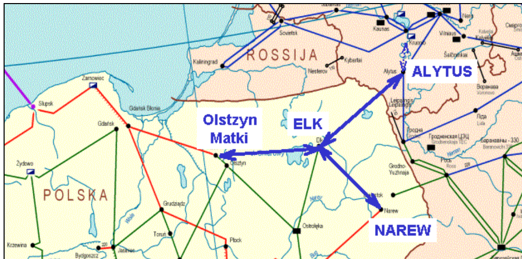
Figure 29: AC-Link between Poland and Lithuania with Back-to-Back Station (500/1000 MW)
