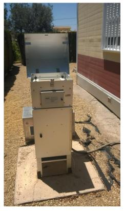
Figure 10. CIEMAT medium volume air sampler
