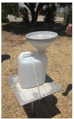
*Figure 11. Atmospheric deposition collector*
