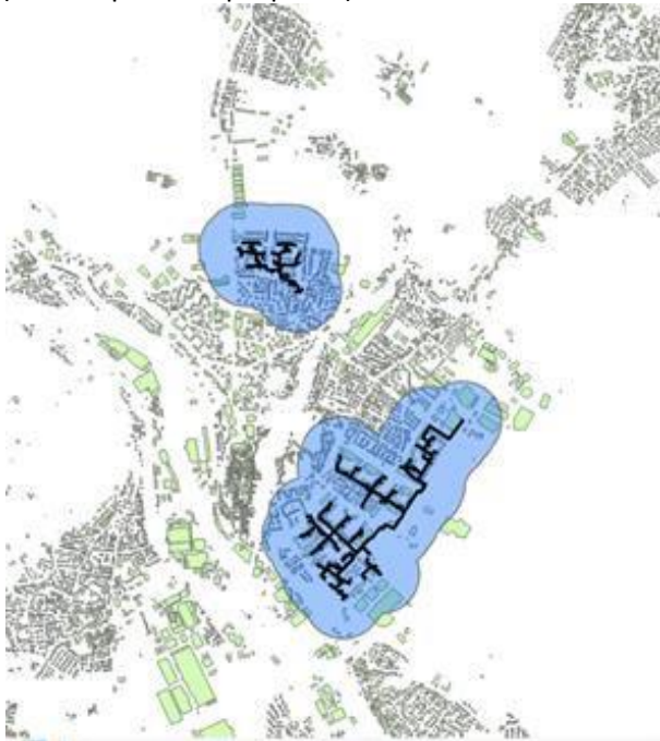
Figure 69: Analysis of the potential expansion of existing DHS using the even expansion approach
