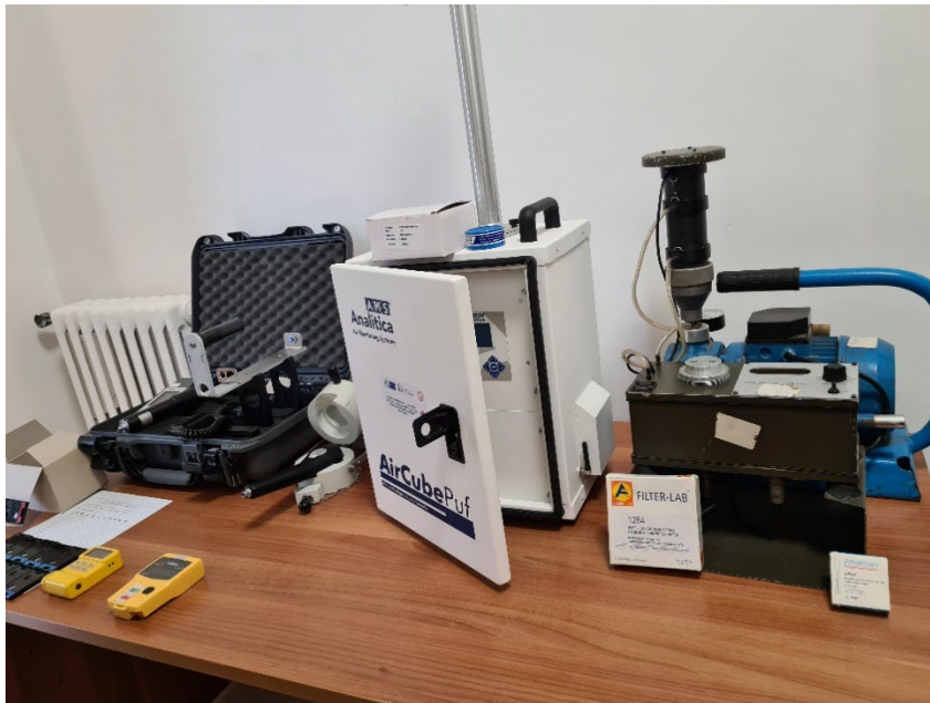
Figure 21. CBRN centre mobile radiation monitoring equipment
