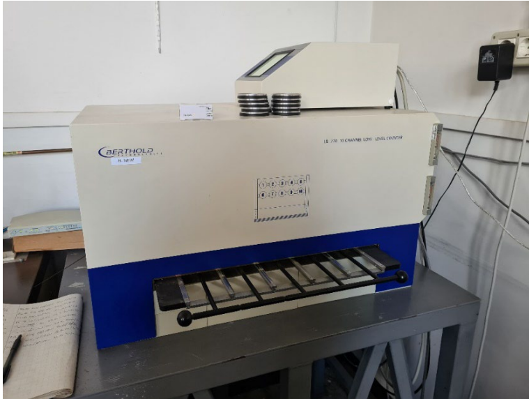
Figure 34. Alpha/beta low-level counter at the ENEA Casaccia Research Centre
