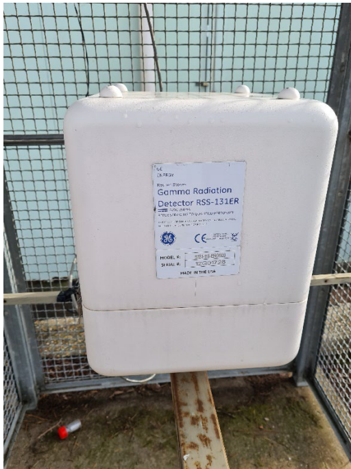
Figure 37. Gamma dose rate monitor at the ENEA Casaccia Research Centre
