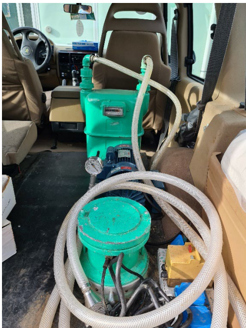
Figure 38. Air sampler in the emergency vehicle at the ENEA laboratory
