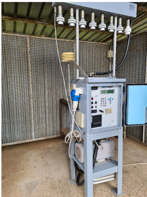
Figure 35. Air sampler 'Capanna'
