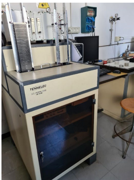
Figure 33. Automatic alpha/beta counter for measuring air filters at the ENEA Casaccia Research Centre
