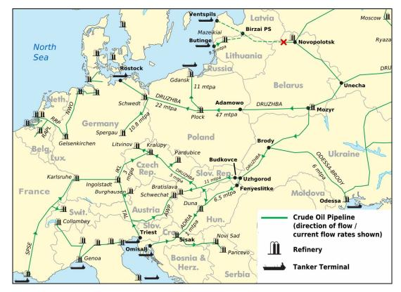
Figure 2-1: Current Flows in Central and Eastern Europe's Oil Pipeline Network
