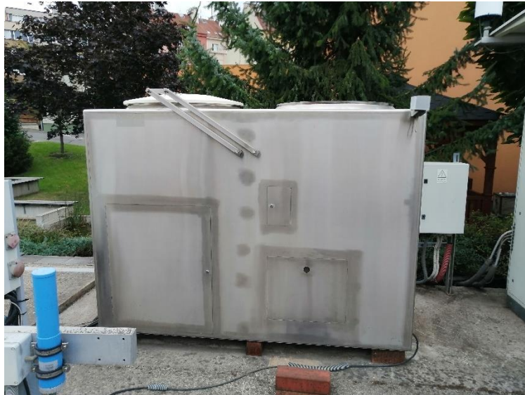
Figure 18. Automatic dry/wet deposition sampler (Pirkko) at SÚRO. The blue detector on the left side is a dose rate monitor part of the national network described in Chapter 7.5.1
