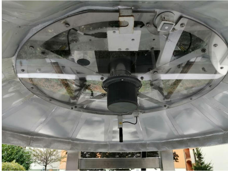
Figure 17. Detector mounted on top of the high-volume sampler air filter
