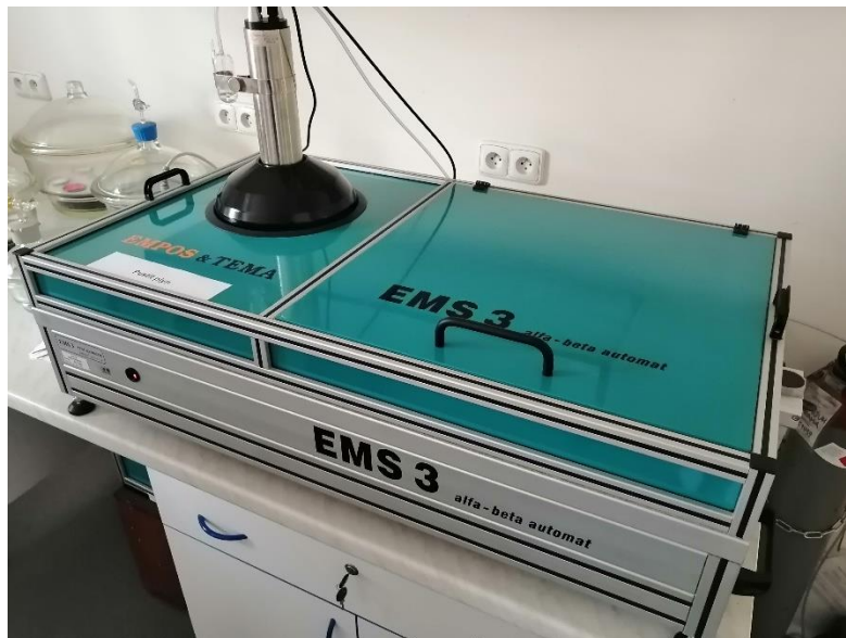
Figure 12. Automatic proportional counter for total alpha and beta counting at the T.G. Masaryk Water Research Institute
