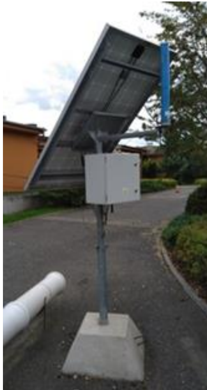
Figure 10. MOSTAR standalone dose rate monitoring station
