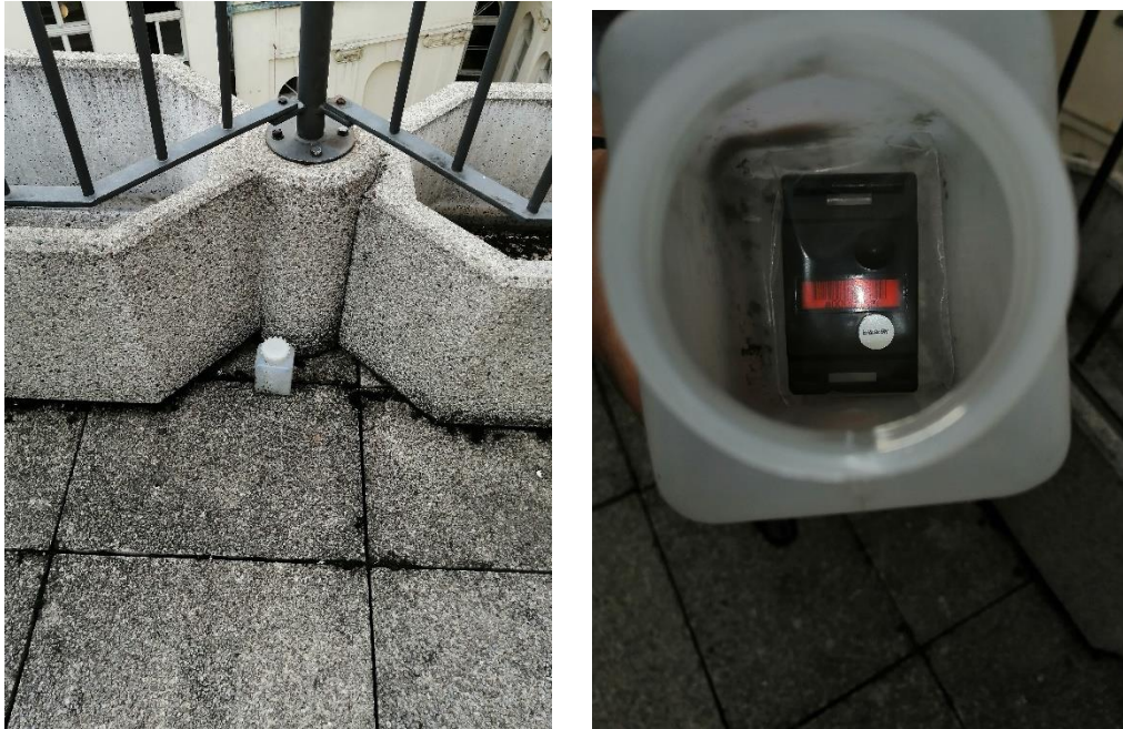
Figure 22. TLD in a plastic container at the SÚJB office roof
