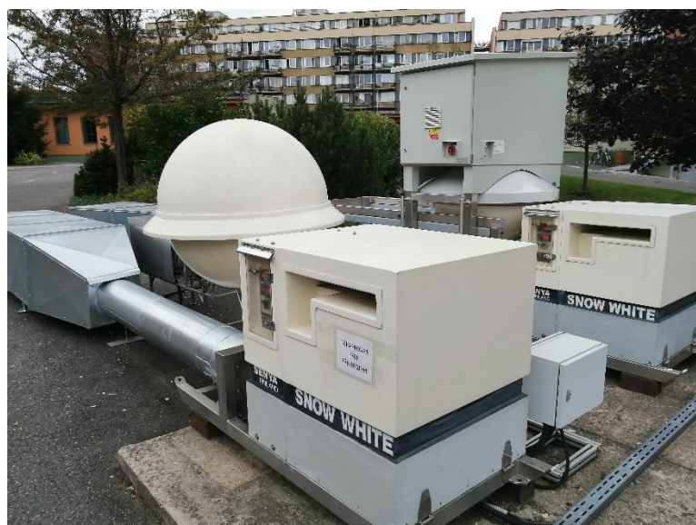
Figure 16. High-volume air samplers at SÚRO
