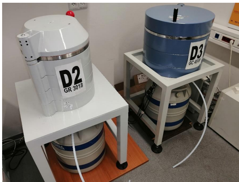
Figure 13. HPGe-detectors at the T.G. Masaryk Water Research Institute
