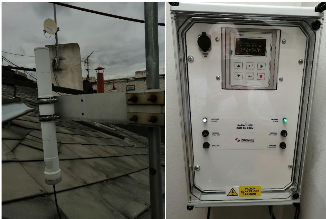
Figure 21. Early warning network station at the SÚJB office roof (left side) and its electronics unit located indoors (right side)
