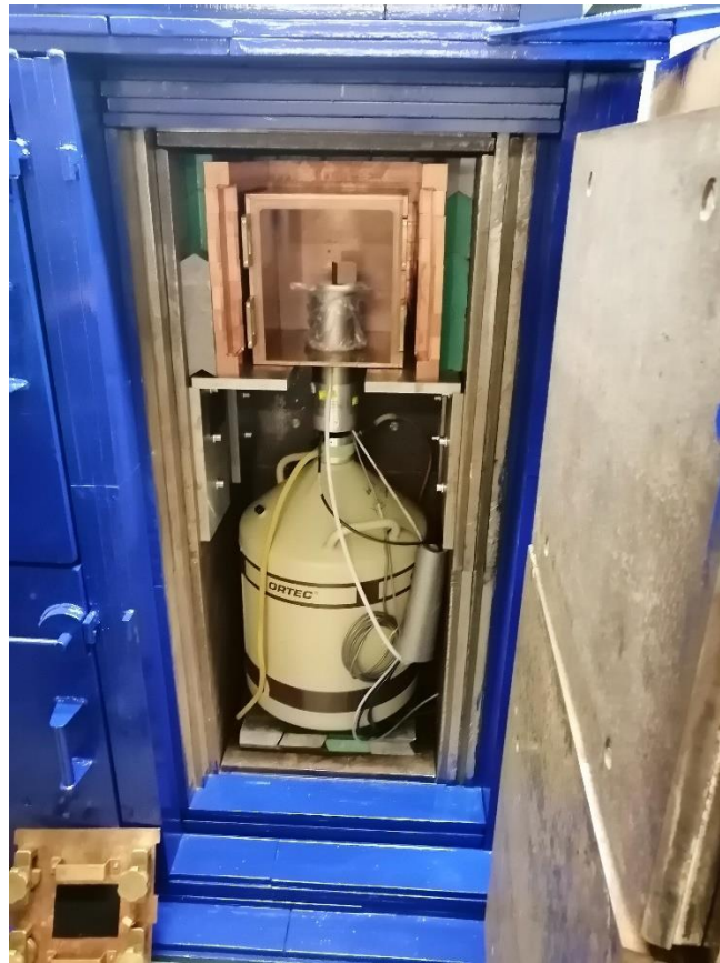
Figure 14. Heavily shielded HPGe detector at SÚRO
