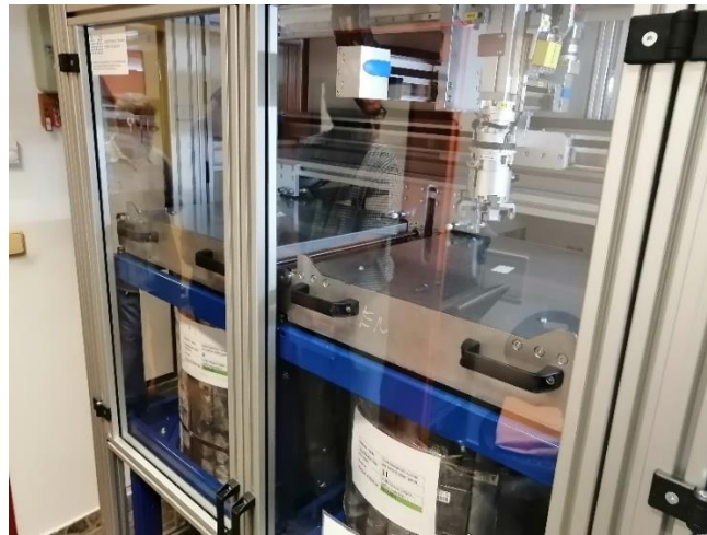
Figure 15. Automatic HPGe analysis system at SÚRO
