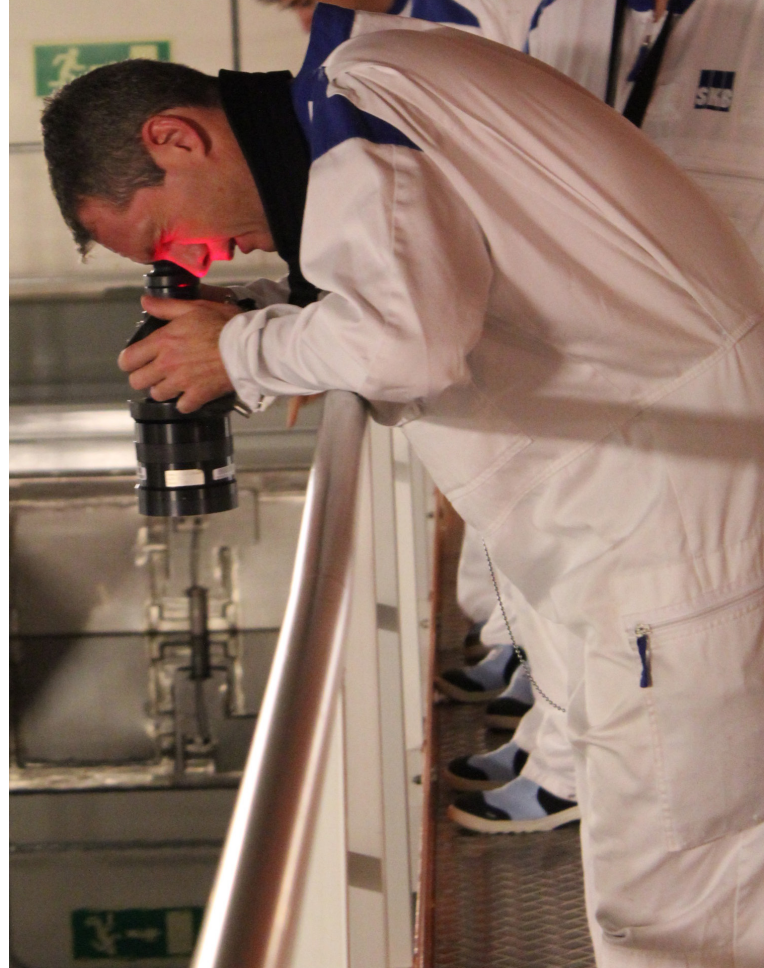
Verifying spent fuel with a Cerenkov Viewing Device
