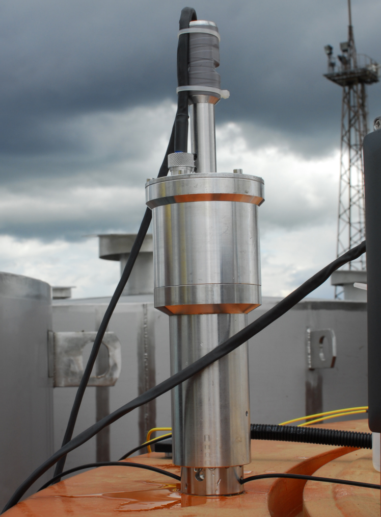
Reading an ultra-sonic seal bolt
