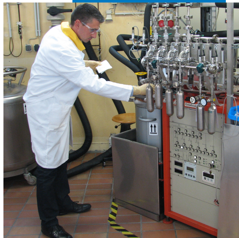
High Performance Trace Analysis sampling at an enrichment plant
