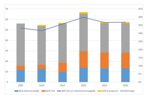
Figure 14. Share of RE in the final energy consumption (right axis – %) and indicative development projections of the share of RE until 2030 (left axis – PJ)<sup>56</sup>
