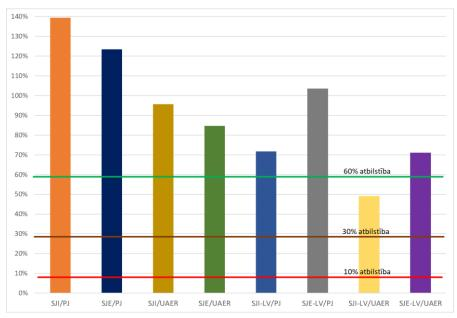
Figure 26. Electricity interconnectivity level of Latvia in 2018
