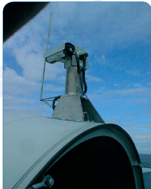
CleverFarm: Outside mounted camera with pan, tilt and zoom. (Camera: Overspeed GmbH)
