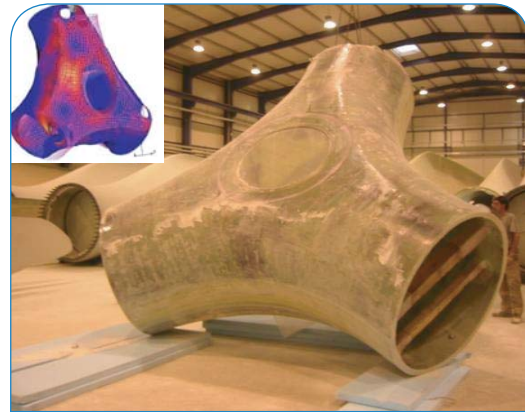
COMHUB: manufactured composite hub.
