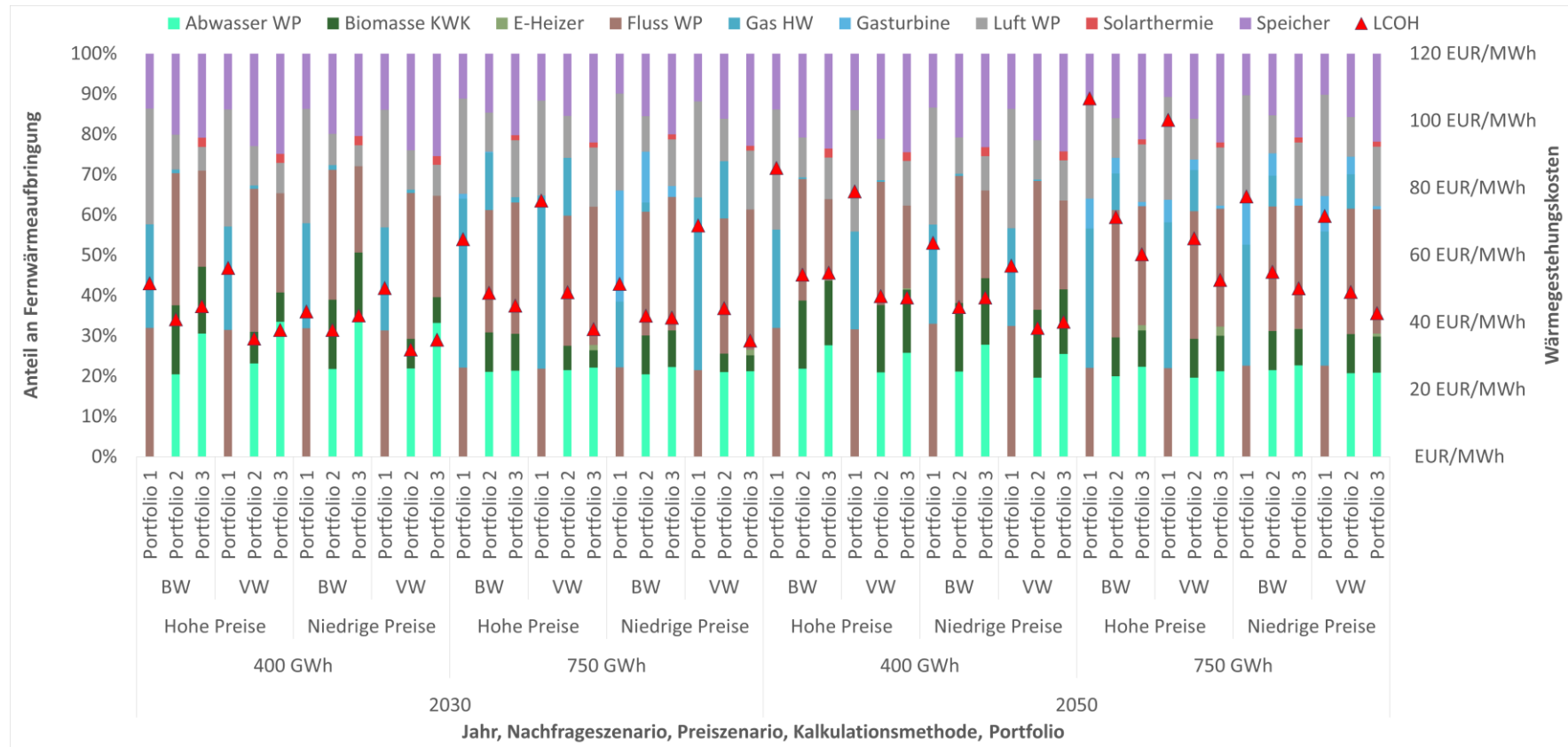
Figure 22: Share of different technologies in district heating generation and the resulting heat generation costs for the Cluster 7 example
