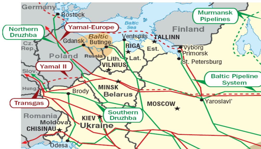
Figure 3-22 The Baltic Pipeline System, gas pipelines shown in red color, oil pipelines in green and the dashed line shows the planned pipelines (source: EIA)
