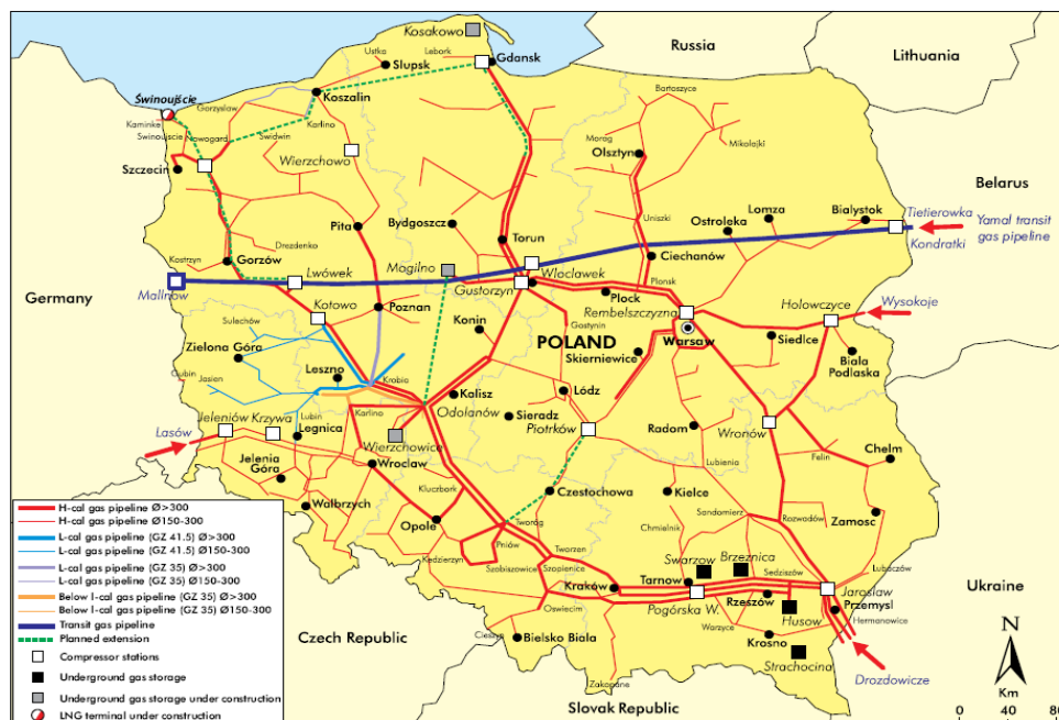
Figure 3-66 Gas Infrastructure of Poland (source IEA 40 )
