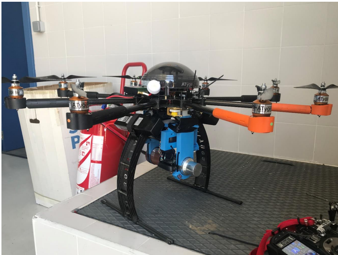
Figure 10. LARUEX radioactivity monitoring drone
