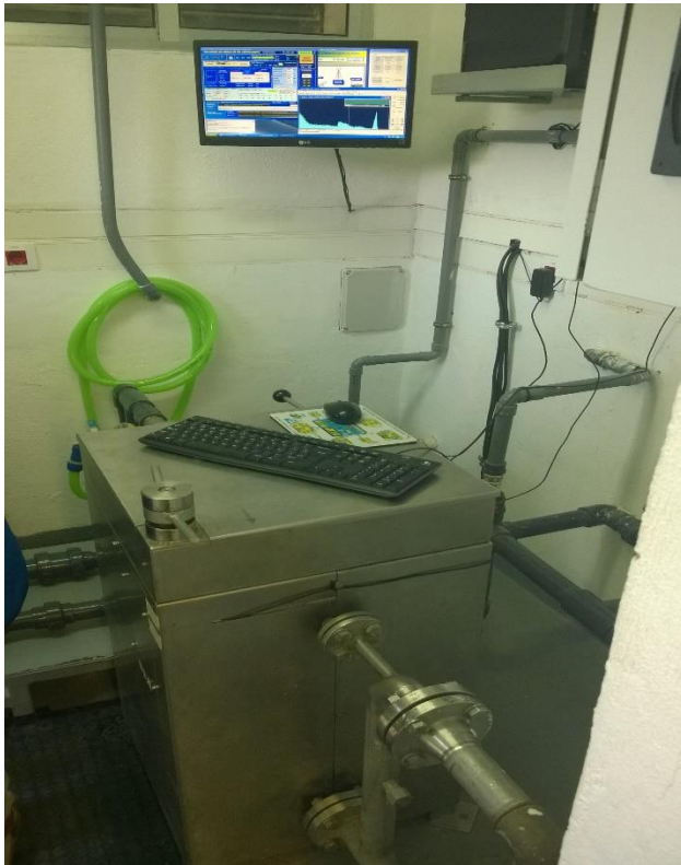
Figure 9. RARE continuous water radioactivity monitor for the cooling water discharge to river Tajo
