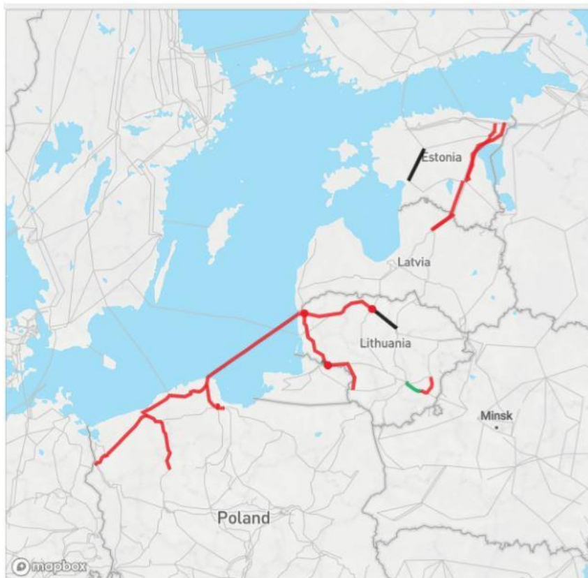
Figure 11: Synchronisation of the Baltic electricity system with the Continental European frequency band 62 . The figure shows the preliminary draft of the synchronisation plan and covers the updated lines.
