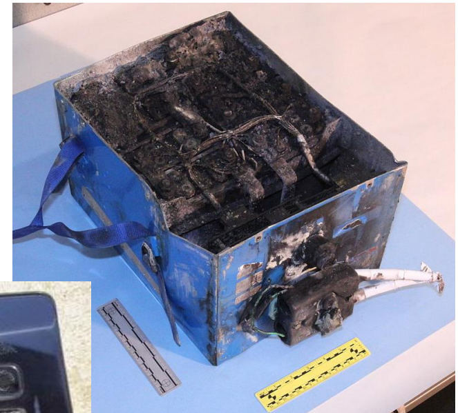
Boeing Dreamliner after internal short circuit ( https://en.wikipedia.org/wiki )
