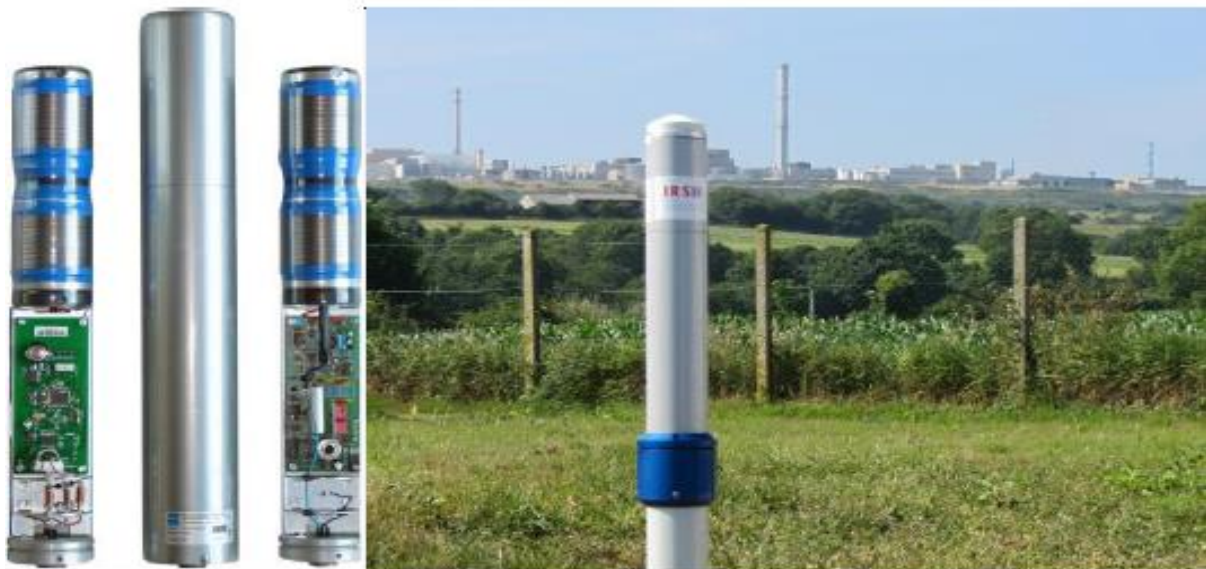
Figure 2. BITT Technology detectors used by the IRSN
