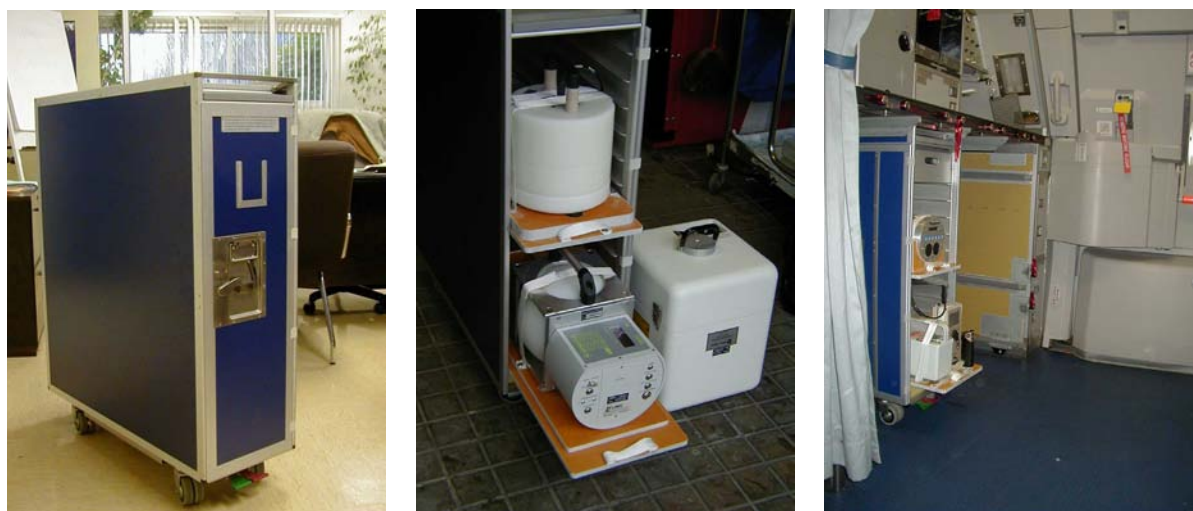
Figure 2: Installation of the instruments on-board: Left: Modified aviation trolley; Middle: Compensated neutron rem-meters and Pressure Ion Chamber (Center); Right: Trolley fixed in the forward galley in an Airbus-340 aircraft.
