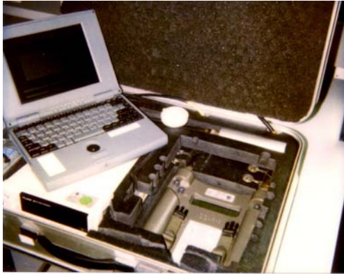
Fig. A10.1: High integrated and transportable measurement equipment for measuring the non neutron component using an external GM-detector and a PC controlled data acquisition system.
