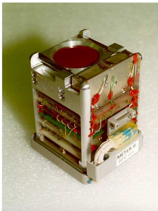
Fig. A.8.1 DOSTEL as flown on Shuttle Missions and in airlight altitudes
