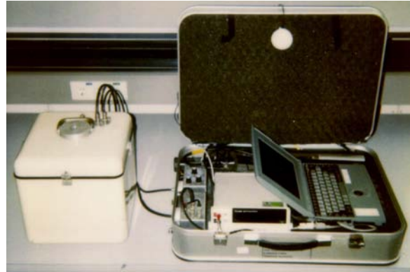
Fig.A10. 2: The high pressure ionization chamber works at 2.5 MPa of argon gas, active volume of 8000 cm 3 for measuring the non neutron component. The data acquisition unit is installed in an easy transportable bag. The white disk in the top of the bag cover shows the GPS antenna.
