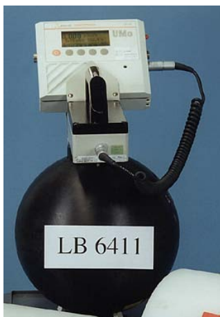
Fig.A10.3: Dosimeter for the neutron component: The LB (marked by LB 6411) is a spherical rem counter specifically tailored to correctly measure H*(10) in the entire energy region from thermal to 20 MeV.
