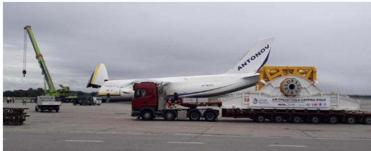
Subsea Well Response Project Capping Stack, in Norway (air freightable)
