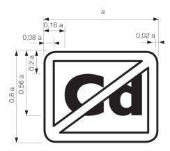
The dimension of "a" shall be greater than 9 mm and the typeface to be used is 'Gill Sans'.
