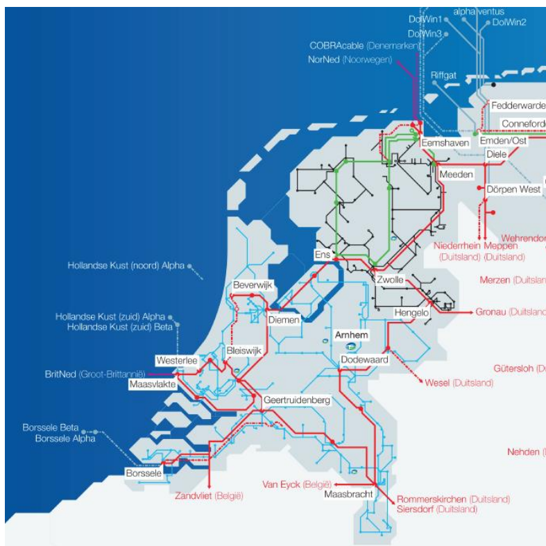
Figure 4.18 Transmission network and interconnectors (Source: TenneT)
