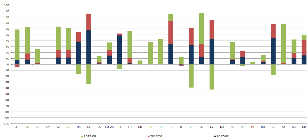
Figure 3 - Deviation of actual Heating Degree Days (HDDs) from the long-term average, in July-September 2017
