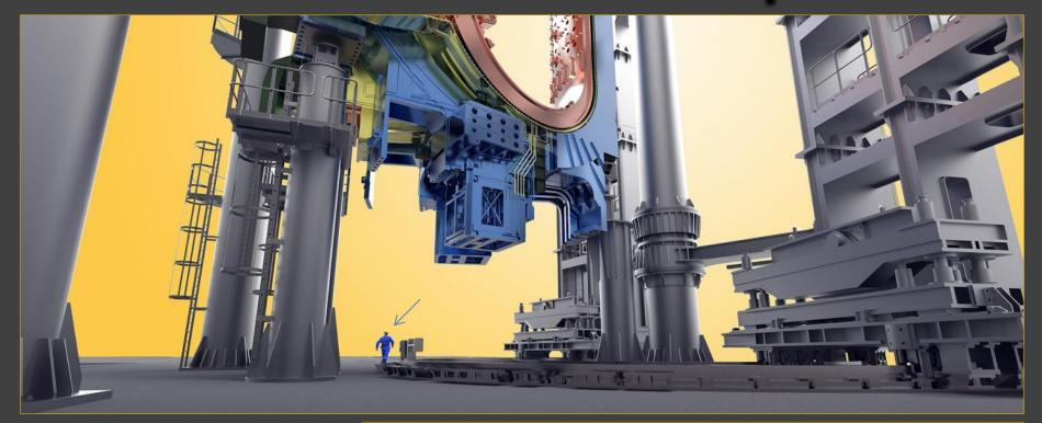
Inside the Assembly Hall, giant tools will handle loads up to 1,500 tons
