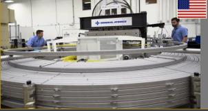
• 1,000-ton Central Solenoid fabrication on-going
