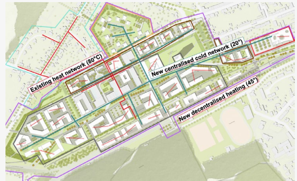
FIGURE 33: HEAT AND COLD SUPPLY CONCEPT FOR THE NEW WESTERHOLT COLLIERY TRANSITION AREA, GERMANY.
