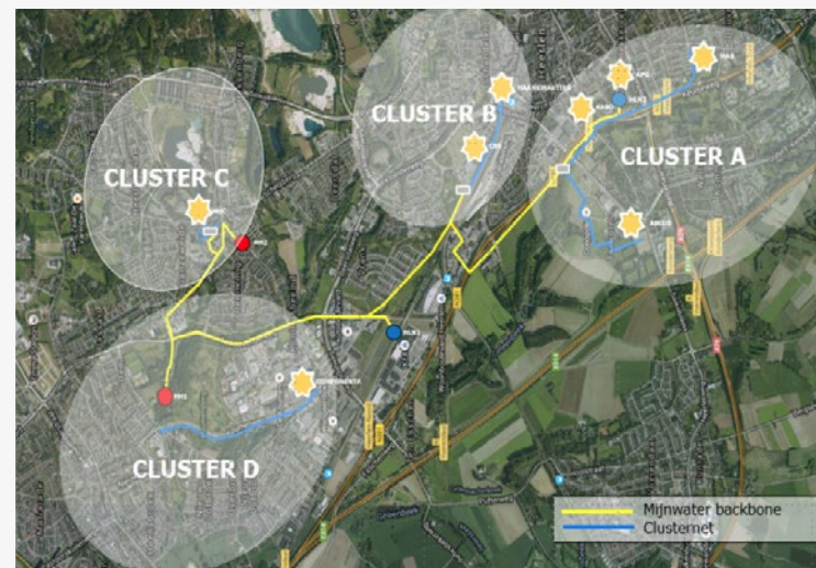
FIGURE 32: A MAP OF HEERLEN MUNICIPALITY SHOWING THE CLUSTERS, PIPE NETWORK AND HOT & COLD DRILLING WELLS, THE LATTER INDICATED BY RED AND BLUE DOTS.
