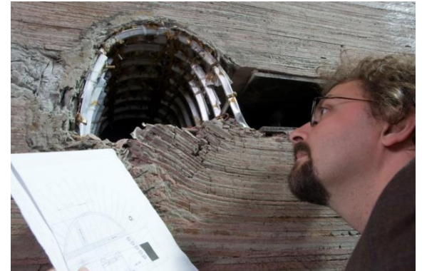
Physical modelling of stresses around a roadway in an underground coal mine
