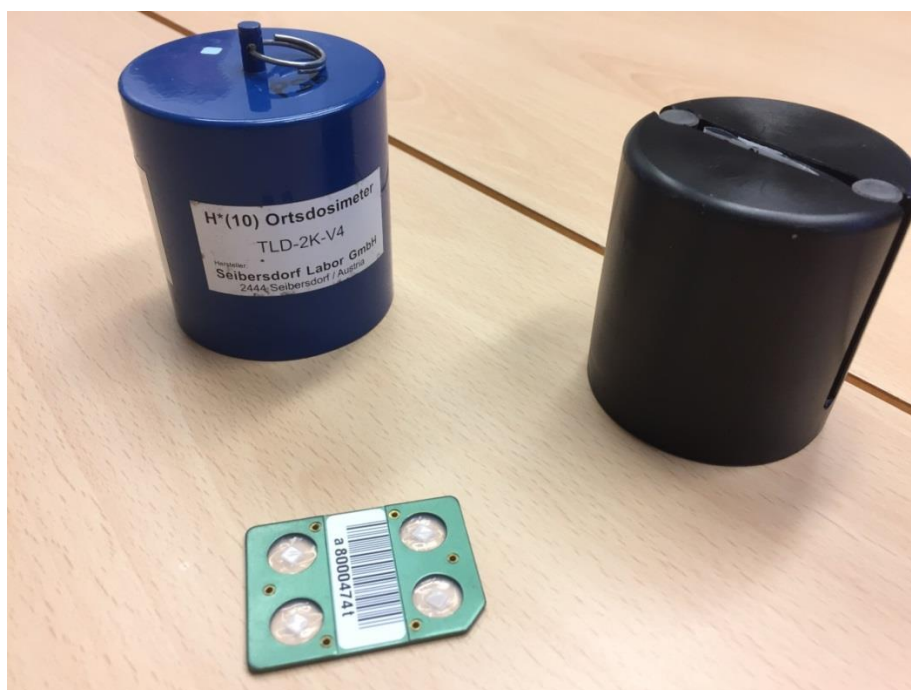
Figure 8. TLD dosimeter and its Seibersdorf holder for environmental dose monitoring
