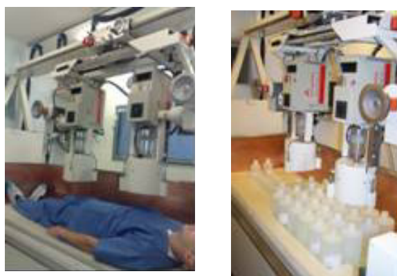
Figure 1 In vivo measurement and efficiency calibration using a physical (bottle) phantom in the mobile in vivo counting laboratory of IRSN
