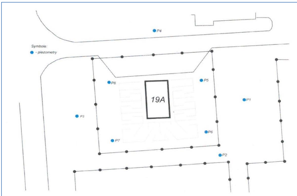
Figure 12: Groundwater sampling points in the vicinity of the spent fuel storage facility No 19A
