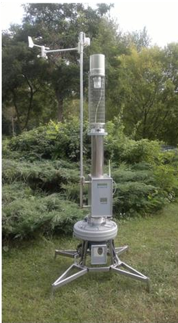
Figure 20: Mobile aerosol sampling station (MASS-1000)
